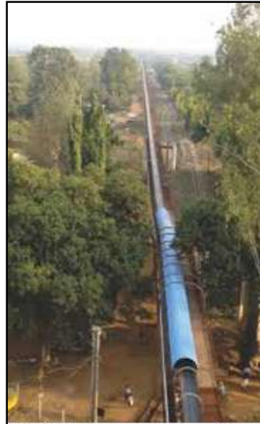
Lime Stone transportation on conveyor belt to OCL Industries PVT. Ltd. Rajgangpur
