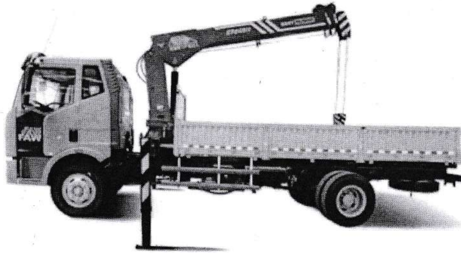
Truck Mounted Crane, GVW 12 Ton with Lifting Capacity 3 Ton
